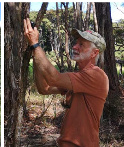
Brian Bramell, MWP's Chair, positions a listening device attached to a bat logger - near the Te Muri Stream. Data will be downloaded weekly and recorded to DOC's Bat Database.
