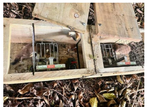
Above: Mike Neil, pest control coordinator and trapping innovator. Below: A modified double trap with double the catch of stoats.
